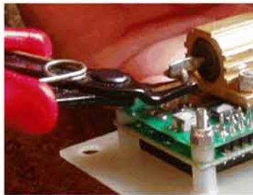
Step 5 Cut resistor link to PCB (opposite end to leads).
