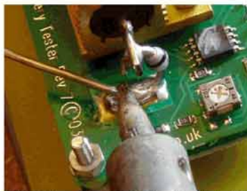
Step 8 Solder Diode link into position (black band to resistor).
